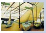
Here, timber was left to season for at least five years. The various types of boat constructed in these shipyards included the nav, a craft of 8 metres in length and 2.7 metres in width, with a 7.5-metre mast. The boat was propelled by four oars and a hemp sail.
